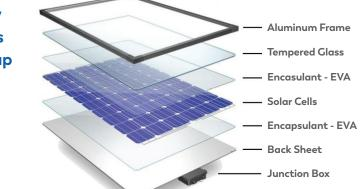
Of these sandwiched layers, the majority (approximately 96%) of the PV module is made up of glass, aluminum, and polymers.
